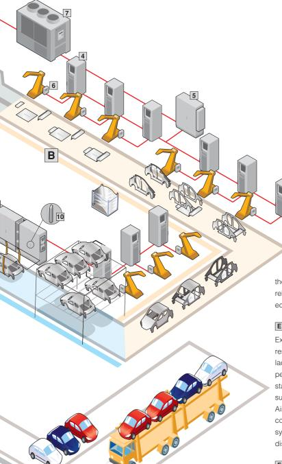
systems – the individual steps are combined into a process chain. Precise, stable handling calls for complex control, for which TS 8 enclosure suites (8) with climate control (9) and access security (10) represent the core.
